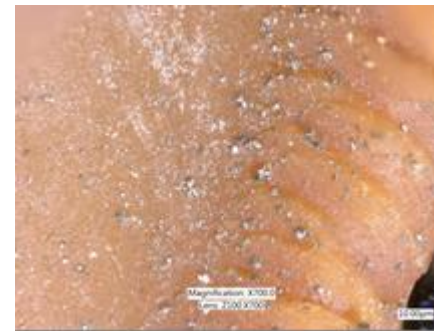
Failed valve seal
