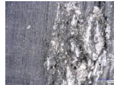
Failed rider band
