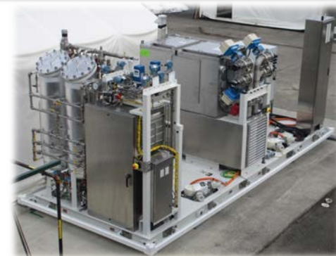
200 kW SOFC System BOP
