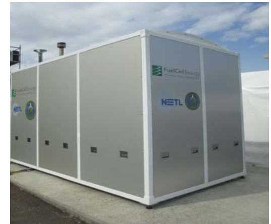
50 kW System: Natural Gas Fuel (8'x20'x8'6")
