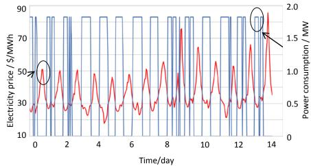
Example of cost-optimized operation of hydrogen electrolyzer that accounts for the dynamic price of electricity (using time-of-use electricity prices) Accomplishments and Progress: Scenario definition sub-model: FCEV adoption and hydrogen refueling station deployment
