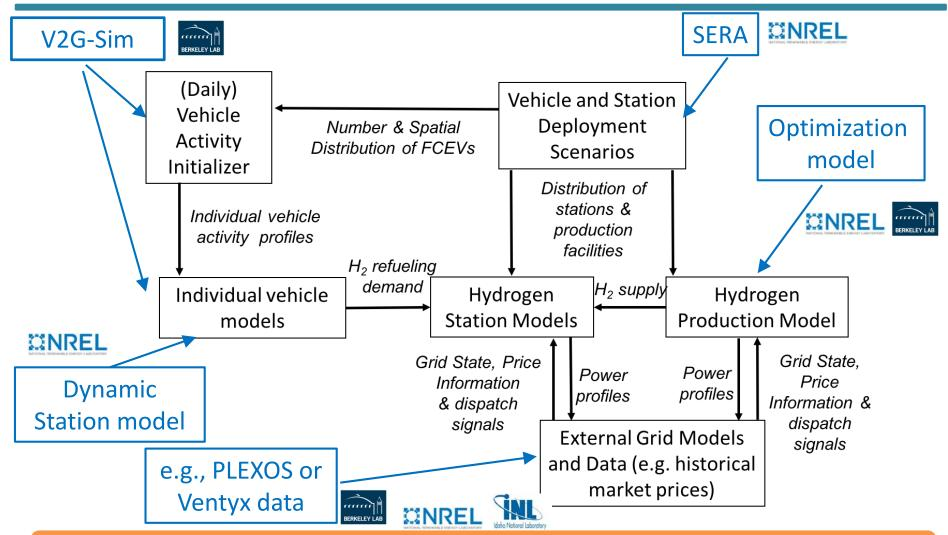
The H2VGI model integrates multiple operational and deployment models for FCEVs and H2 generation resources with external grid models across various time scales
