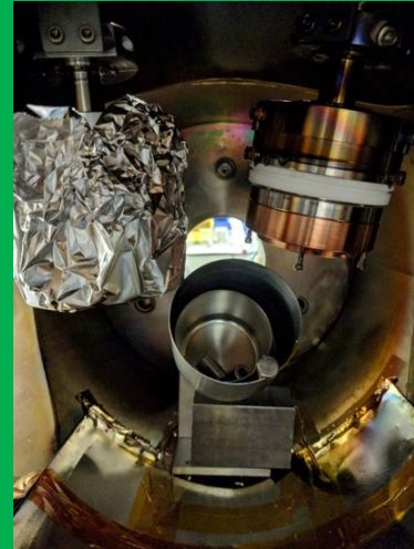
DC magnetron sputtering chamber at Oak Ridge National Laboratory (small batch)
