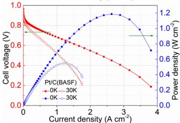
AST condition: Voltage cycling from 0.6 V to 1.0 V @ 50 mV/sec, Anode =  $\text{H}_2$  @ 100% RH, Cathode =  $\text{N}_2$  @ 100% RH, Temperature = 80 °C, P = 100 kPa
