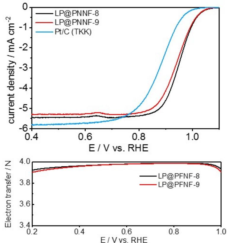
ORR catalytic activities were measured by RRDE method in O<sub>2</sub> saturated HClO<sub>4</sub> (0.1M) at RT;
