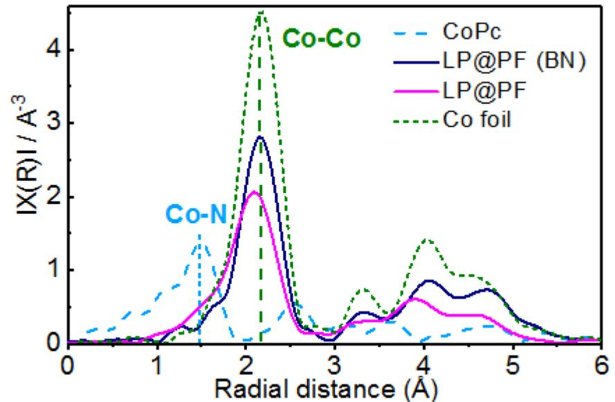
**X-ray absorption spectroscopies identified formation of additional PGM-free catalytic sites over the “support” during the post-treatment, enhancing the synergistic catalysis**
