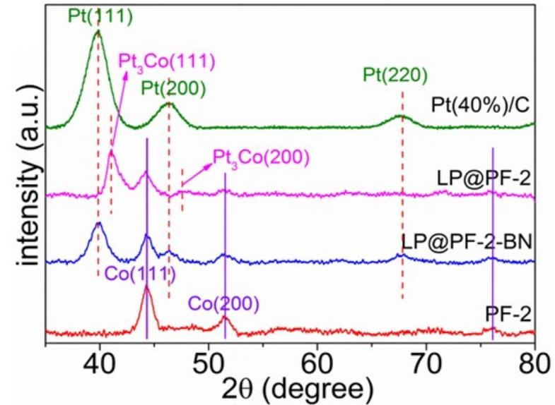
**XPS and XRD further confirm the Pt-TM NP alloy formation and distribution of carbonaceous nitrogen during in situ reduction**
