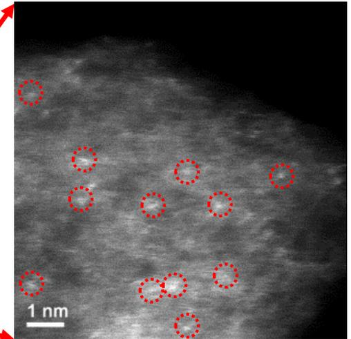
Atomic Co is embedded in N/C composite in PGM-free substrate
