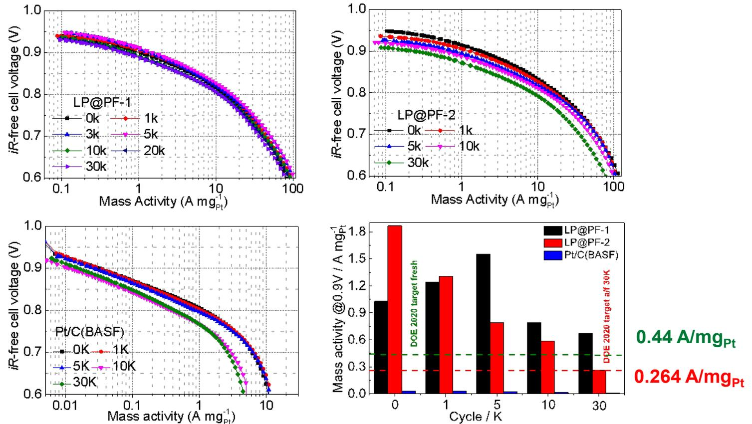
Although performance loss was observed during AST, the mass activities of both LP@PF catalysts still met or exceeded 0.264  $A/mg_{Pt}$ , or 60% of initial 0.44  $A/mg_{Pt}$  of DOE 2020 target at the end of 30 K cycles
