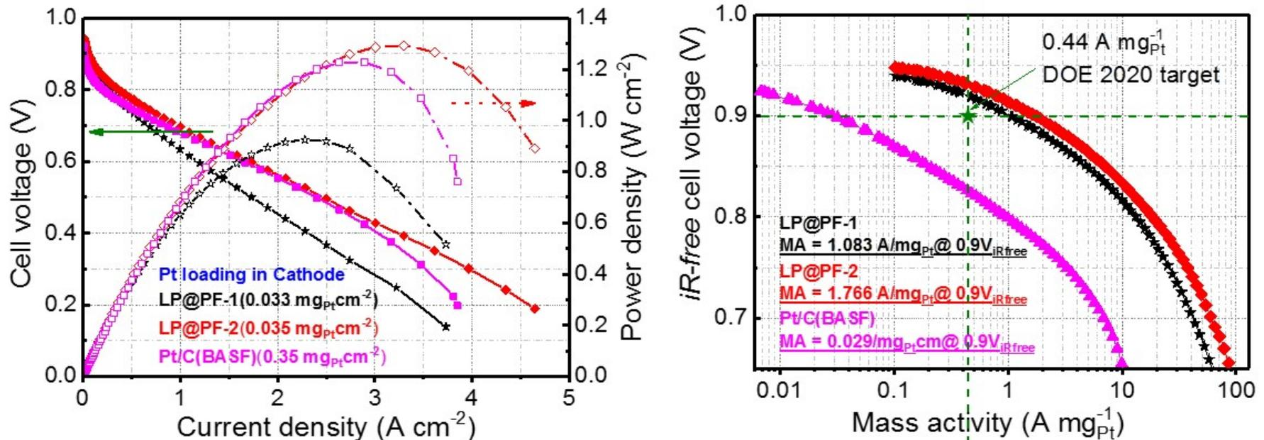
Test condition: membrane = Nafion 211, Temperature = 80 °C, P<sub>H<sub>2</sub></sub> = P<sub>O<sub>2</sub></sub> = 100 kPa @ 100% relative humidity (RH) (back pressure = 50 kPa), flow rate = 200 mL min<sup>-1</sup>
