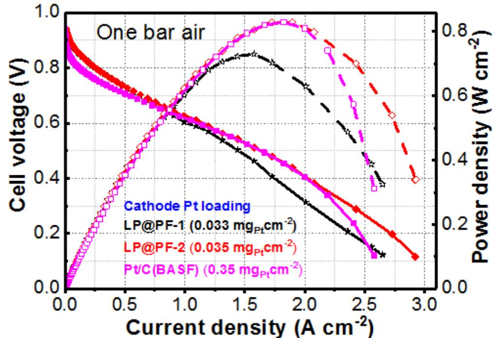
Test condition: membrane = Nafion 211, Temperature = 80 °C, P<sub>H<sub>2</sub></sub> = P<sub>AIR</sub> = 100 kPa @ 100% relative humidity (RH) (back pressure = 50 kPa), flow rate = 1000 mL min<sup>-1</sup>.
