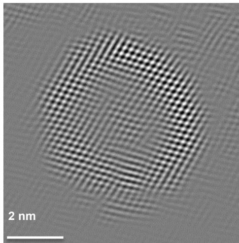
Pt-Co alloy NPs are situated over Co/N<sub>x</sub>/C<sub>y</sub> catalytic support
