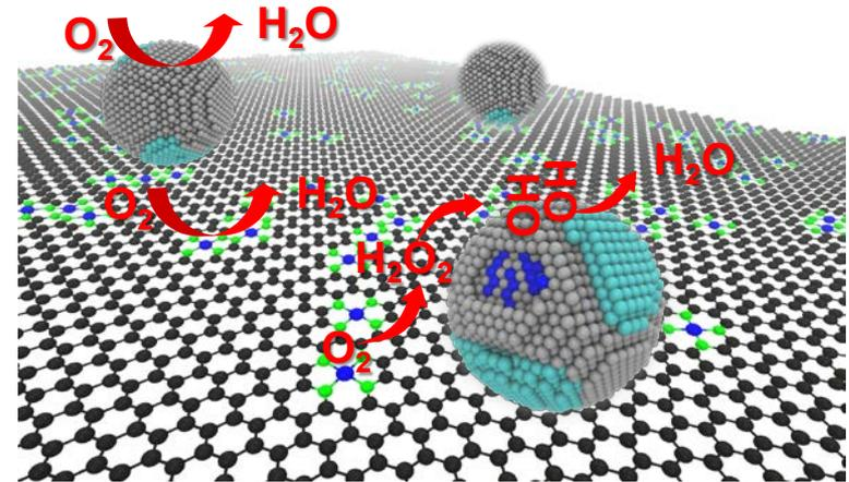
*In addition to parallel catalysis at both sites, sequential reactions between PGM-free and Pt sites improve overall kinetics:*
