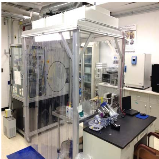
Beneq TFS500 – up to 20" 3D chamber, larger substrates, scale-up
