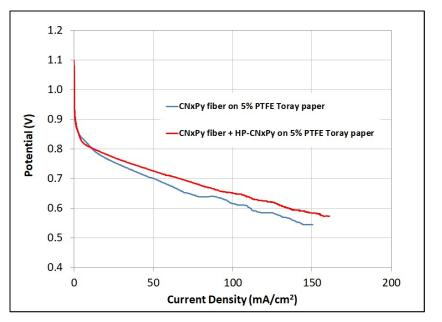
Improved performance with the addition of 5-wt% surface-treated hydrophobic additive in the catalyst layer for alkaline fuel cell testing
