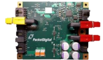
Power Management and Distribution Board
