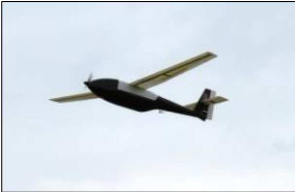
Ion Tiger PEM Fuel Cell UAV
