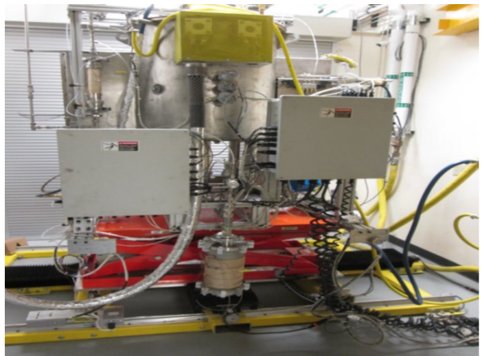
CU hybrid receiver (back showing xyz stand, etc.)
