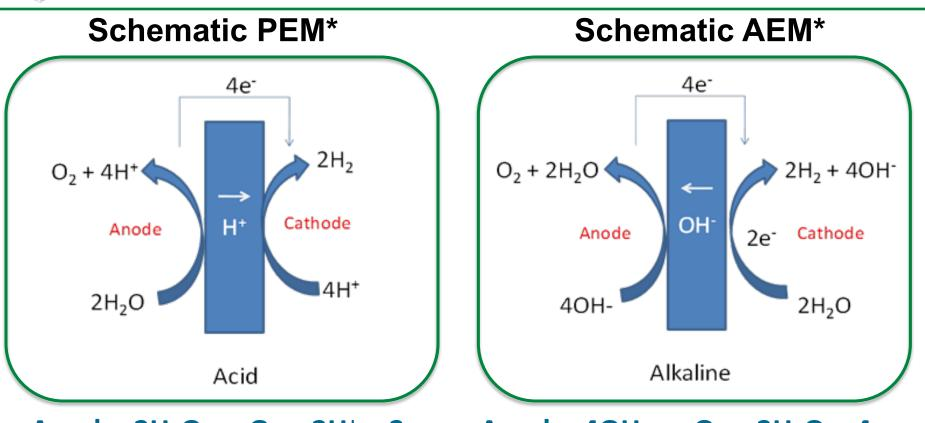
Anode:  $2H_2O => O_2 + 2H^+ + 2e^-$ Cathode:  $2H^+ + 2e^- => H_2$
