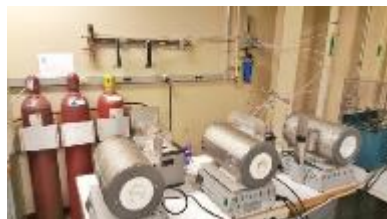
Metal alloy selection: oxidation rig at LBNL
