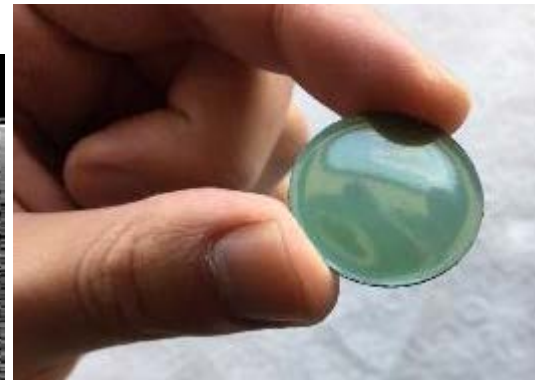
Anode-supported cell with YSZ electrolyte
