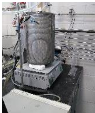
Four-probe Conductivity Test setup Assembled at UConn
