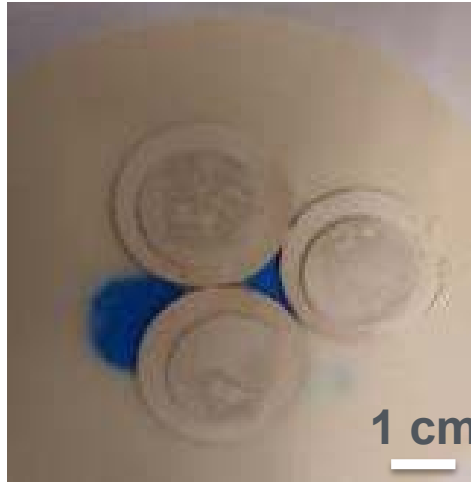
BZY, BZCY-Yb pellet by isostatic pressing (1.6 cm diameter)
