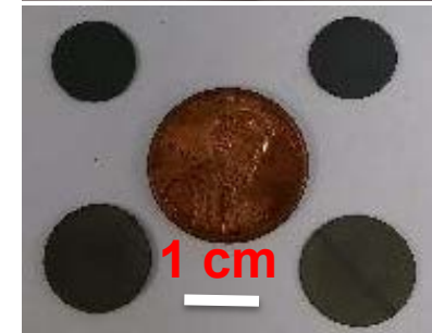
Dense BZY and BZCY-Yb electrolyte (~1.3 cm diameter)
