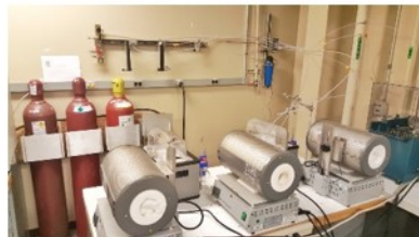
Metal alloy selection: oxidation rig at LBNL
