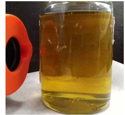
Steam electrode precursors in solvent (25g Toluene + 10g IPA + 5g ethanol)
