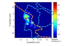
Photoluminescence image shows no degradation of the perovskite under 2layers of MoS<sub>2</sub>
