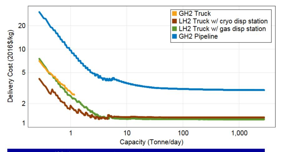
Delivery costs (\$/kg) as a function of capacity for each delivery technology and refueling station type assuming a 5 km delivery distance (transmission costs not included) Within conventional pathways above, LH2 distribution outcompetes other modes.
