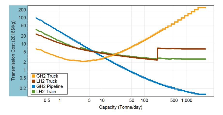
Transmission costs of the primary component technologies in the SERA model assuming a transmission distance of 100km.
