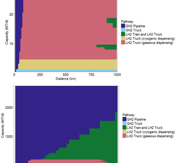
**Contour plot of lowest cost** pathways for relatively low capacity (top) and high capacity (bottom) hydrogen supply-chain from the point of production to the retail station.
