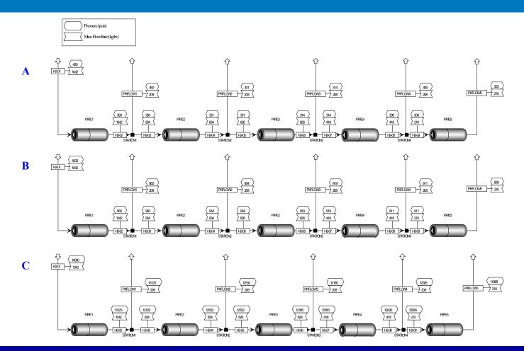
ASPEN modeling of hydrogen pipeline sizing for: (A) 400 psi pipeline inlet pressure (flow is from left to right), (B) 1,000 psi pipeline inlet, and (C) 14,000 psi pipeline inlet. Pipeline inner diameter corresponding with A, B, C scenarios is 3.6 in, 3.0 in, and 1.0 in, respectively.
