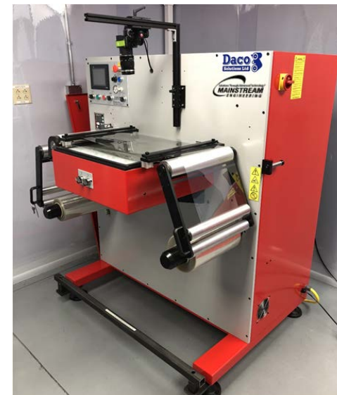
R2R film inspection station with Automated Dynamics machine vision system commissioned February 28
