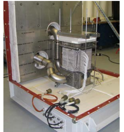
Example of a thermally self-sustained stack module design
