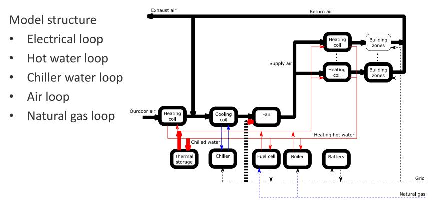
Additional equipment needed for different building types can be added into appropriate loop as well as novel configuration.
