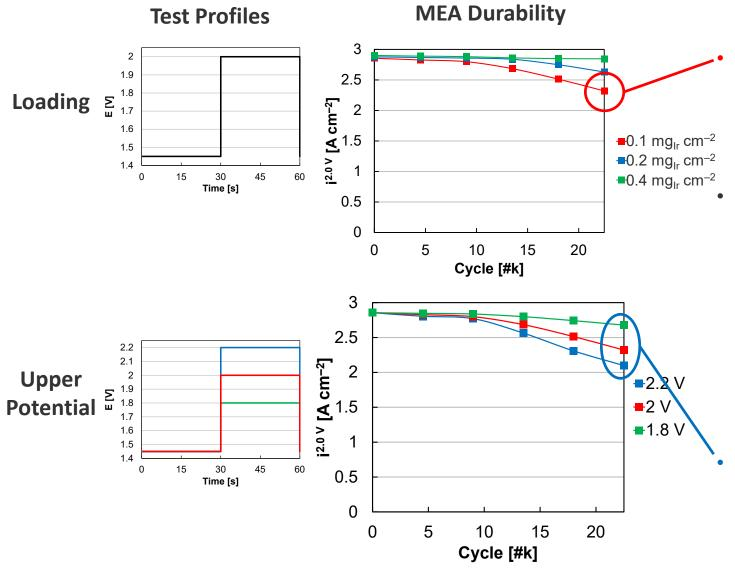
Low loading required to see durability losses during short time frame
