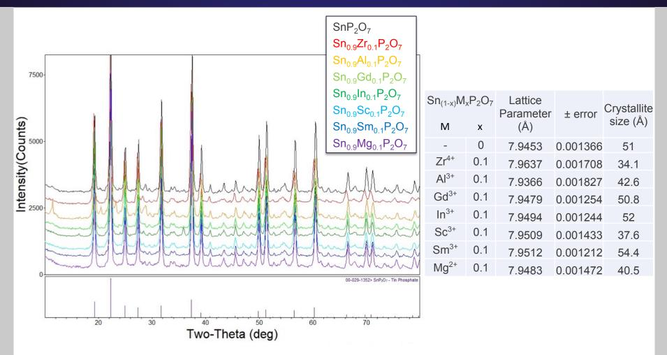
Synthesized Sn<sub>1-x</sub>M<sub>x</sub>P<sub>2</sub>O<sub>7</sub> powders with aliovalent dopants and varying amounts of excess polyphosphate phase
