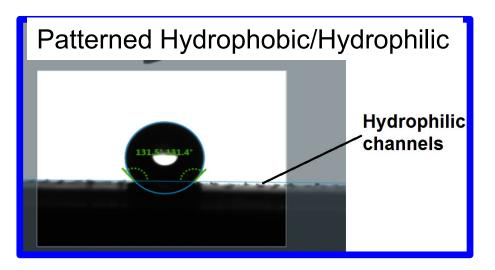
Hydrophobic/hydrophilic patterning maintains high bulk hydrophobicity of GDL, while still providing local water transport pathways
