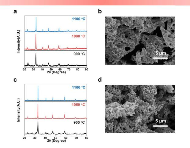
Positive electrodes (NBSCF, and PBSCF) with desired perovskite phase has been synthesized by solution combustion method;
