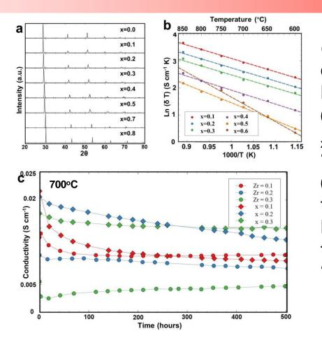
(a) XRD patterns at room temperature obtained for the synthesized  $BaM_xCe_{0.8-x}Y_{0.1}Yb_{0.1}O_3$  powders; (b) conductivities of the  $BaM_xCe_{0.8-}$  $_xY_{0.1}Yb_{0.1}O_3$  measured at 600 to 850 °C in wet argon (3 vol% H<sub>2</sub>O); (c) evolution of the conductivities of the  $BaM_xCe_{0.8-x}Y_{0.1}Yb_{0.1}O_3$  and  $BaZr_xCe_{0.8-x}Y_{0.1}Yb_{0.1}O_3$  electrolytes as the function of time measured at 700 °C in 25% CO<sub>2</sub>, 25% H<sub>2</sub>O and 50% H<sub>2</sub>
