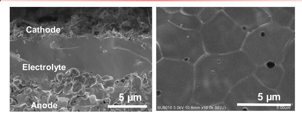
A dense electrolyte with a thickness of ~8 um;
