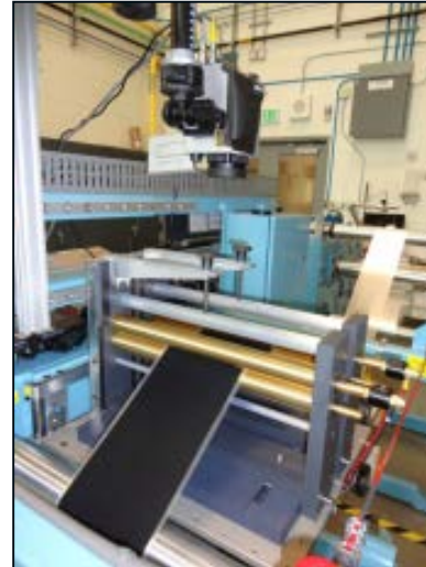
Infrared imaging of electrode and MEA defects
