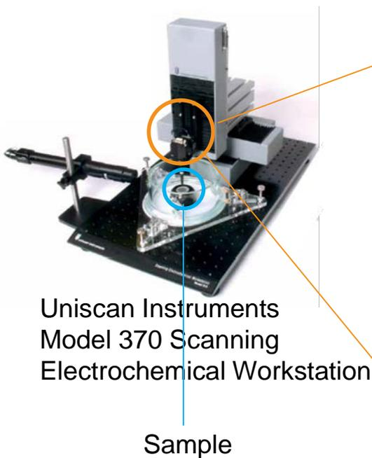
SECM ultramicroelectrode probe for reversible redox reactions
