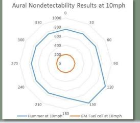
By comparing two like vehicle systems (Colorado ZH2 & HMMWV) the fuel cell vehicle has a 75-90% improvement for its acoustic signature.
