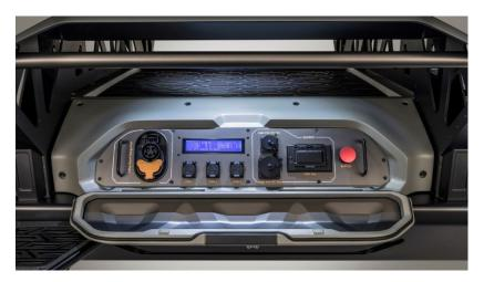
Extended Silent Watch Provides 2.5 kw of export power For 24 hours on 4kg of H2 (~4gal JP-8 equivalent)
