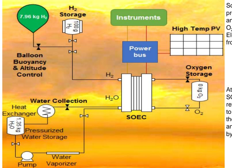
Solar array powers the probe at high altitude and generates  $H_2$  and  $O_2$  with Solid Oxide Electrolysis Cell (SOEC) from stored  $H_2O$
