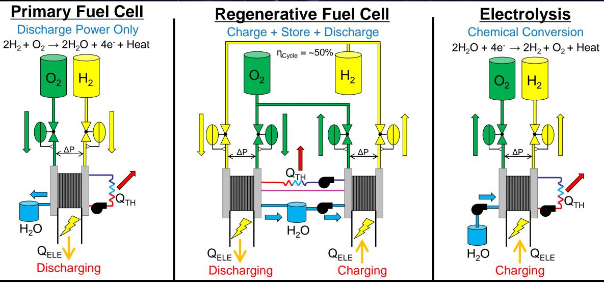
Regenerative Fuel Cell = Fuel Cell + Interconnecting Fluidic System + Electrolysis
