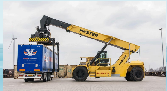
Reach Stacker 80,000 lbs lift capacity
