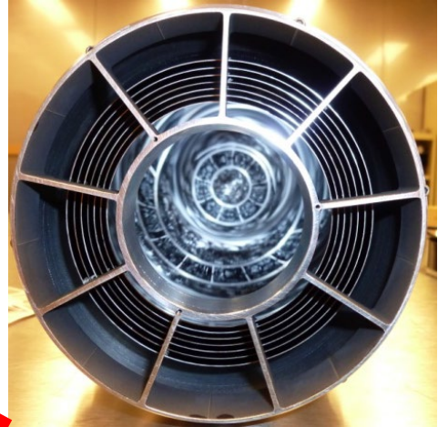
Condenser optic: a standard x-ray telescope (5 shells, 60 cm long, 10 cm diameter) that will concentrate ~1% of guide into objective for 1000 flux
