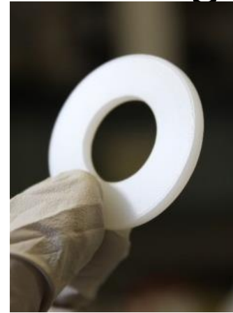
Example of a Hydro-Pac seal received by GVD prior to coating.
