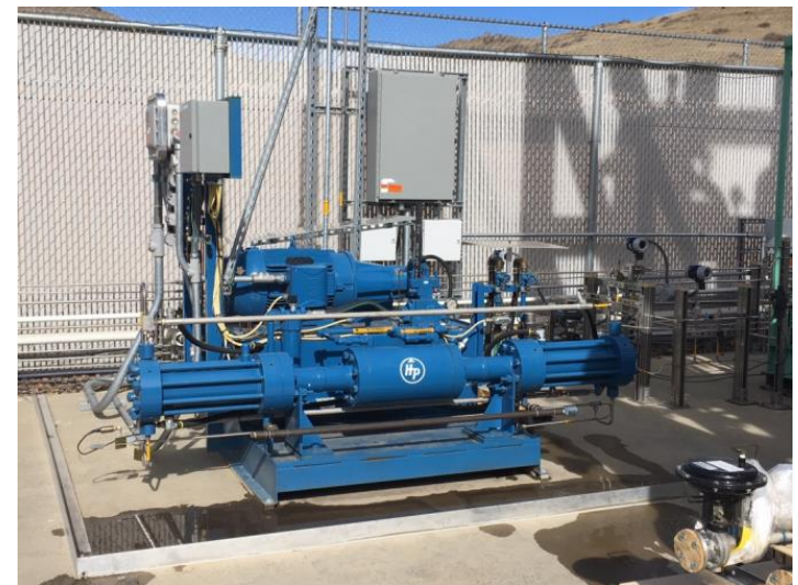
Hydropac compressor similar to that used in NREL testing
