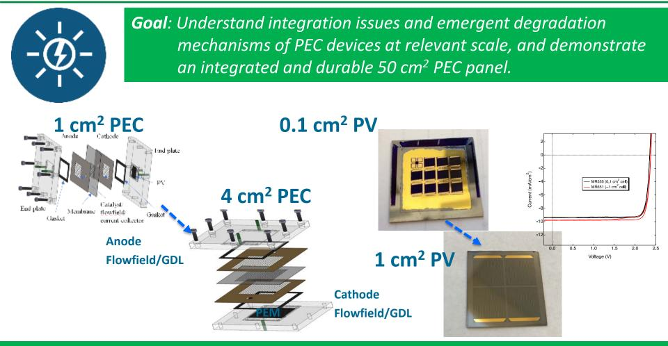
**Accomplishments**: PV fabrication scale up from 0.1 to 1 cm<sup>2</sup> PEC vapor cell scale up from 1 to 4 cm<sup>2</sup> Benchmarking PEC cell performance between NREL and LBNL
