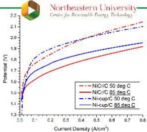
Anode: Ni-Fe/Raney Ni; Membrane: polyaryl piperidinyl triphenyl (PAP-TP-MQN), prepared by University of Delaware (UD)
