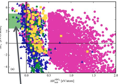
Targeted space: Stable (x<0) and Reduction Suitable for Water Splitting (y between 2.5 to 5 eV)
