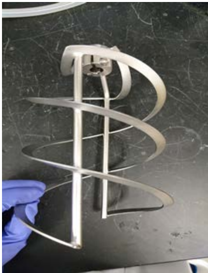
Potential impeller design to be used for high solids bioprocess
