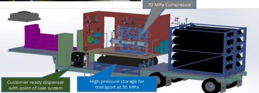
Designed and developed advanced hydrogen mobile fueler (AHMF) capable of fueling approximately 20-40 fuel cell vehicles per day up to 70 MPa with -40 C cooling.
