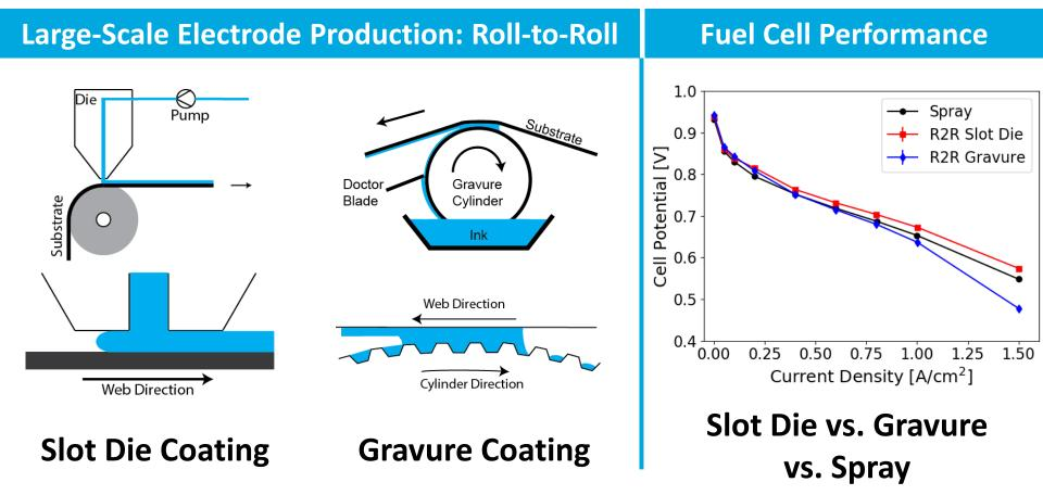
R2R coated gas-diffusion electrode methods are >200x faster than spray coating and the MEAs perform as well.
