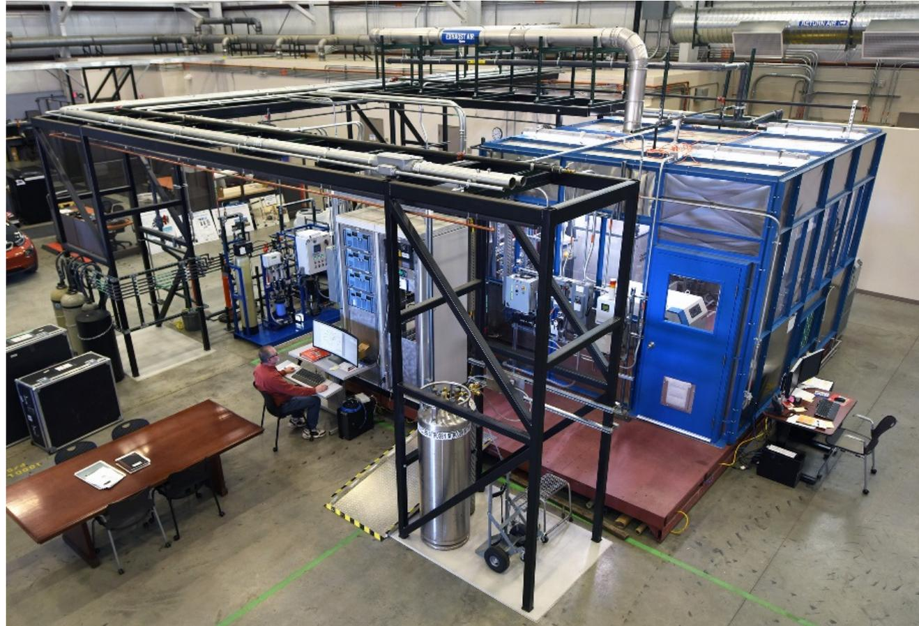
25 kW HTE Test Facility within the INL Energy Systems Laboratory
