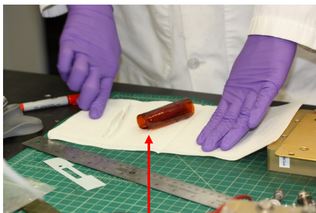
PBI membranes prepared by LANL researchers with 5, 10, and 15% H 2 PO 4 .
