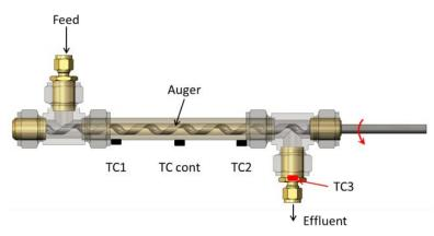
Flow-through reactor design used to validate the model
