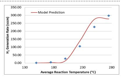
Comparison of model predicted hydrogen flow rate to that measured experimentally for 20 wt% alane slurry
