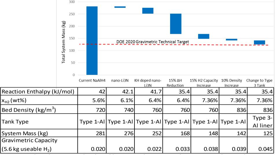
6 nm KH doped nano-Li<sub>3</sub>N developed by Dr. Stavila: Requires larger  $\Delta H_{rxn}$  reduction, but smaller increases in H<sub>2</sub> capacity and density than NaAlH<sub>4</sub> to meet the DOE Gravimetric target
