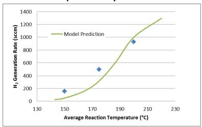
Comparison of model predicted hydrogen flow rate to that measured experimentally for 20 wt% AB slurry
