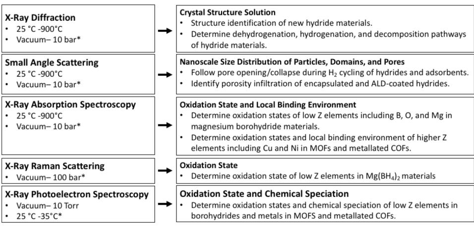
\*Cell development in progress to obtain higher pressures and temperatures
