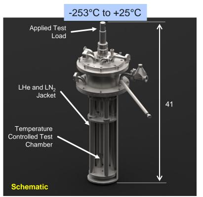
Liquid helium-cooled Janis Research dewar for materials testing with controlled temperature chamber
