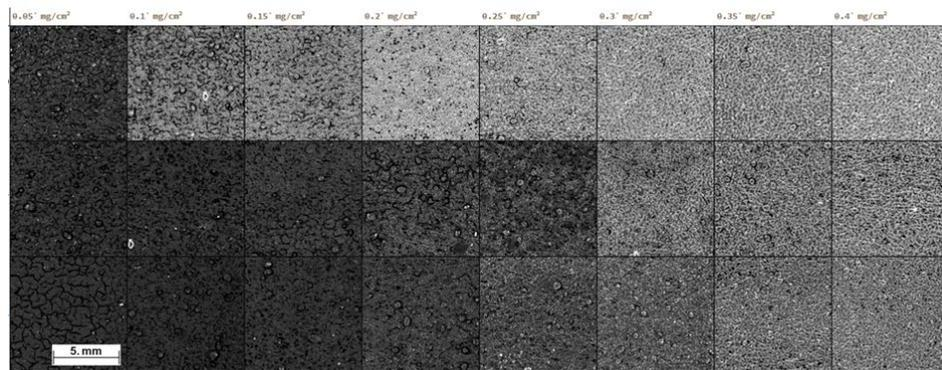
Magnified transmittance images for CCMs indicating differences in macro morphology as a function of loading
