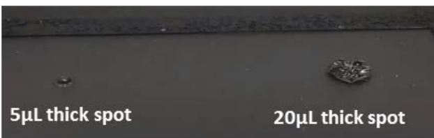
Thick spot fabrication by drop-casting, 3 sizes: 5, 4x 5, 20 µL
