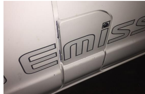
H2 Fueling , Passenger side (fueling location)
