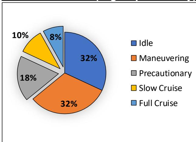
Duty cycle similar to ISO E5 cycle for ferries (emissions test)
