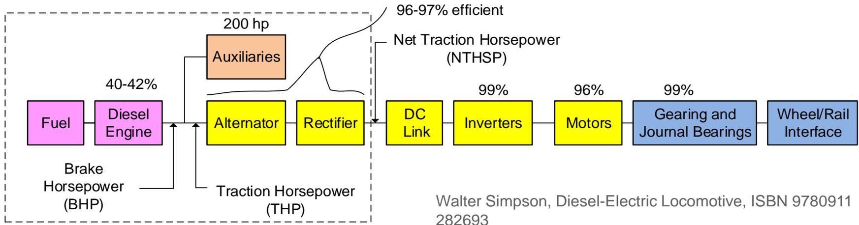
**Replacing diesel engine in an electromotive with FCS is made easier by the existing electric drive. Alternator and rectifier are replaced with a DC/DC converter, offering 2-3% gain in efficiency.**
