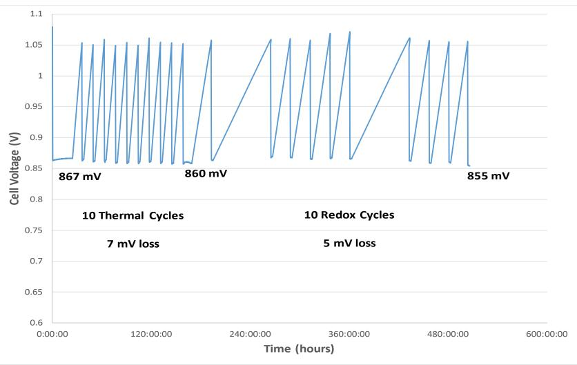
Steady State Hold Results at 750°C over 10 Thermal and 10 Redox Shutdown Cycles With 5 Hour Hot Holds (Fuel Pipes Disconnected)
