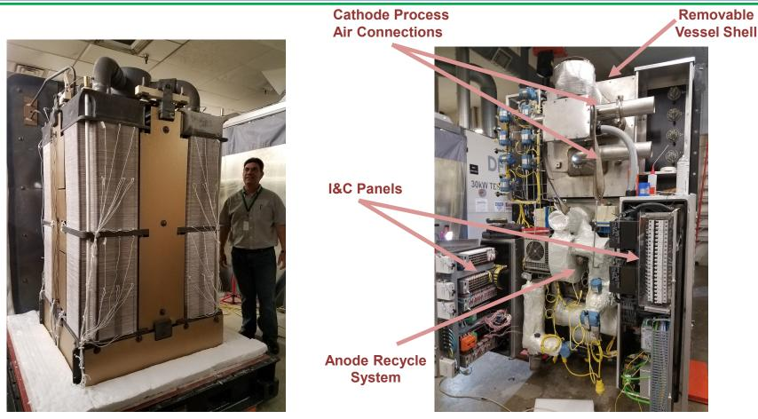
100 kW Stack Module Architecture:
