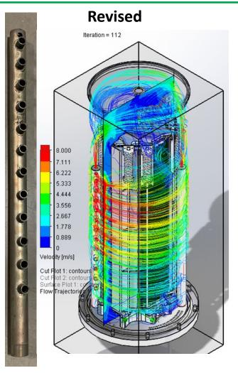
Test results suggested an air flow sensitivity. A re-examination of the air inlet distribution tubes showed a potential cause. Flow momentum at the higher flow rates was favoring air flow to the top. A revised air inlet was designed and built
