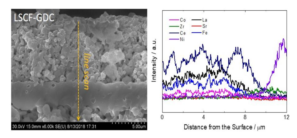
Dense bi-layer electrolyte: ~ 1.7 μm YSZ, 1.0 μm GDC
