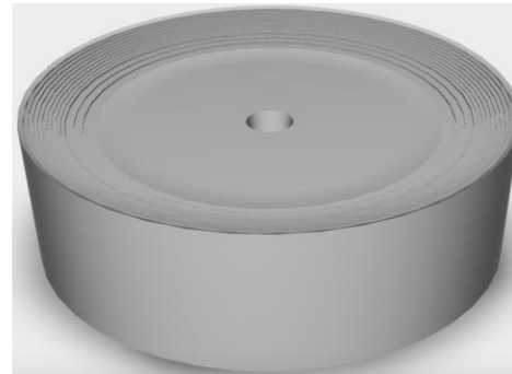
Top of Kovar rotating disk with layered grooves to increase adherence of zirconia coating
