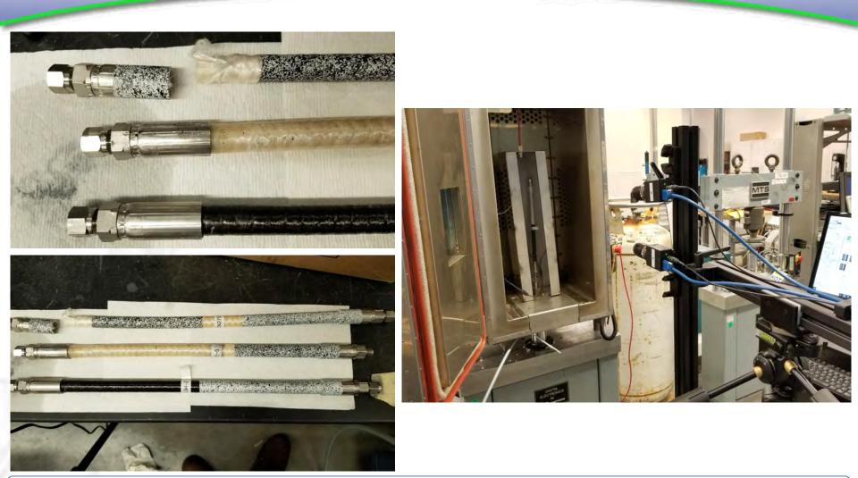
DIC Verified Leakage in Fitting Coupling and 3% strain at Hose/Fitting Interface at 36k psi
