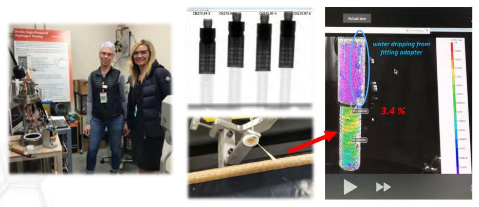
DIC Verified Leakage in Fitting Coupling and 3% strain at Hose/Fitting Interface at 36k psi
