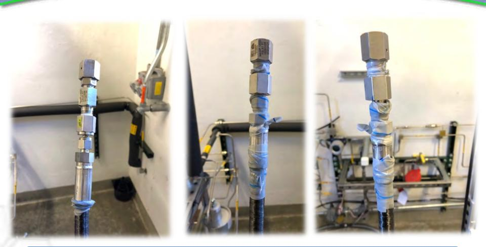
H35 Fills Conducted at NREL with Crimped Fitting rated for 350 bar H<sub>2</sub> Sensing Tape Indicates Leakage at Crimped Areas
