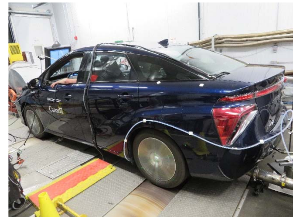
FCEV Exhaust Measurements at Environment Canada (July 2019)
