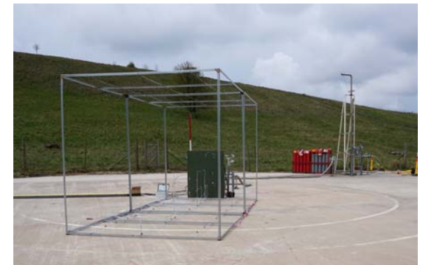
HyWAM support structure down-stream from the HSL LH2 release apparatus
