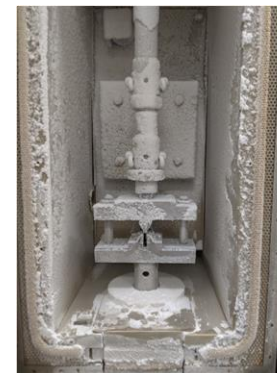
The composite strength increased at lower temperatures (-75°C), but the nanoparticles at the tested concentration did not affect the mechanical strength. So the interlaminar shear strength improvements seen at ambient temperature were not translated to low temperature tests
