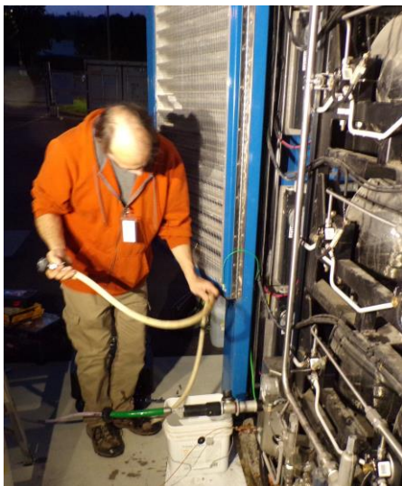
Dave Haywood (Hydrogenics/Cummins) drains old coolant from the MarFC system.
