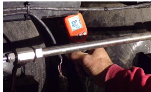
Monitoring MarFC tank temperature during fill.
