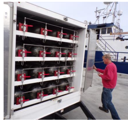
Cascade fill from IGX 350 bar truck tanks
