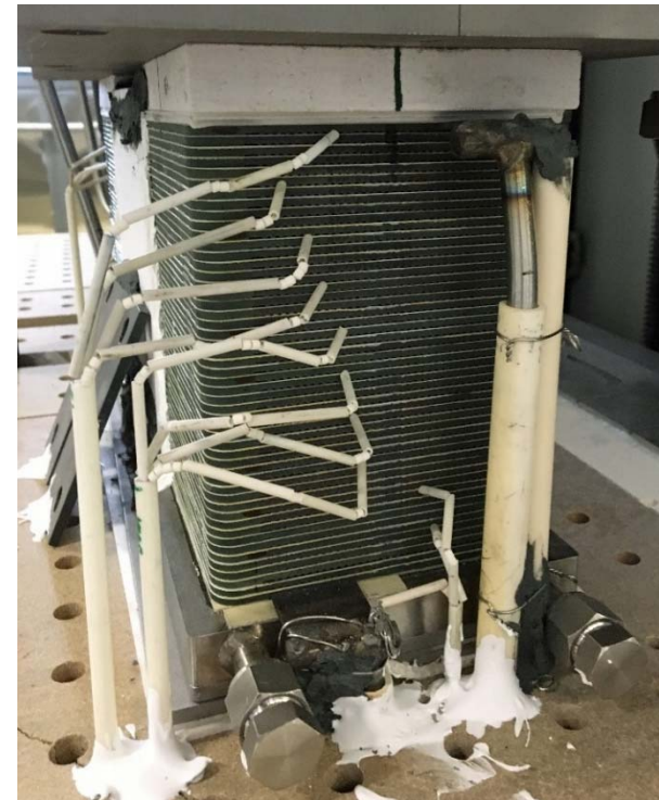
5 kW stack installed in hot zone
