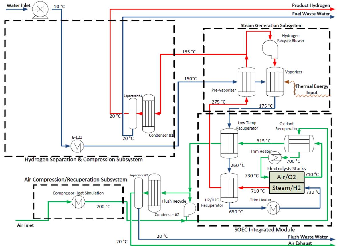
Electrolysis Demonstration System Process Flow Sheet
