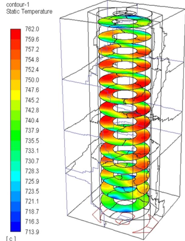
CFD simulations including cell electrochemical performance model is utilized to support CSA stack development
