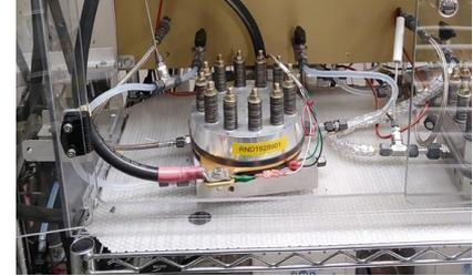
Commercial GDE (#3): Pt 3 mg<sub>Pt</sub>/cm<sup>2</sup> RSDT cathode (#4): Pt/Vulcan XC-72R, 0.2 mg<sub>Pt</sub>/cm<sup>2</sup>, I/C ratio 0.15; RSDT anode, Ir loading, 0.3 mg/cm<sup>2</sup>; RSDT recombination layer: 1X Pt loading, membrane: N117, 50 °C, 400 psi differential pressure; active area: 86 cm<sup>2</sup>.
